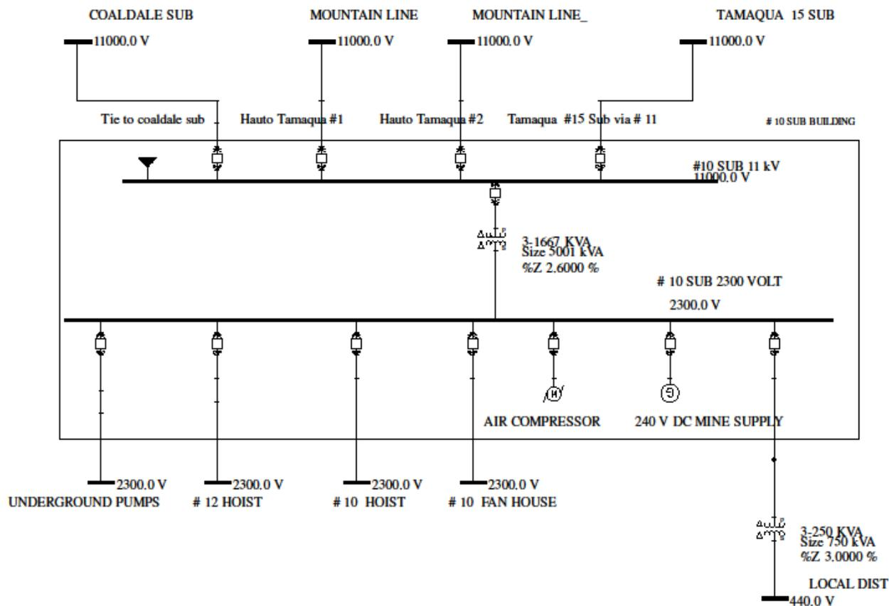
Figure 2 Single Line Diagram of the #10 substation typical design
